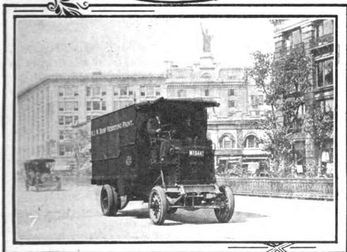
Fig. 6—Large department stores employ a fleet of small wagons for express delivery Fig. 7—Sampson truck with box type of closed body used for heavy work by paint manufacturers
